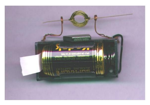
Note that there is a strip of paper stuck in between the battery and the electrical contact in the holder. This is the on/off switch. Remove the paper to allow electricity to flow into the motor, and replace the paper when you want to stop the motor and save the battery.
