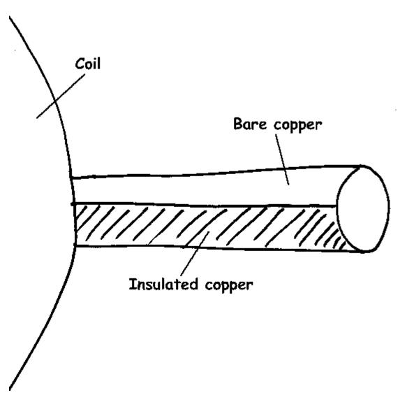
Do the same thing to the other free wire end, making sure that the shiny bare copper side is facing up on both wire ends.
