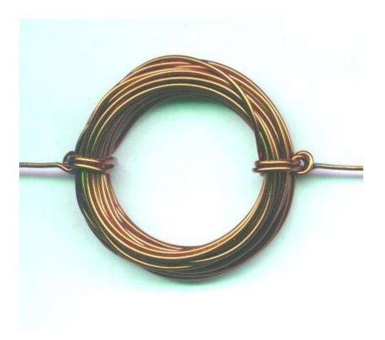
It is not necessary, but I usually wrap a couple turns around these binding turns as well, threading the wire into the space between the large coil and the small coils that hold it together. This makes for a neat, tight package, as in the photo below:
