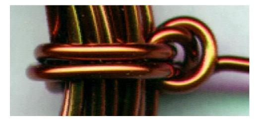
If this method of holding the coil together is too difficult, feel free to use scotch tape or electrical tape to do the job. The important thing is to keep the coil together, and to have the two ends of the wire anchored well, and aligned in a straight line, so they form a good axle.
